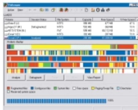
Example of a typically fragmented partition.
